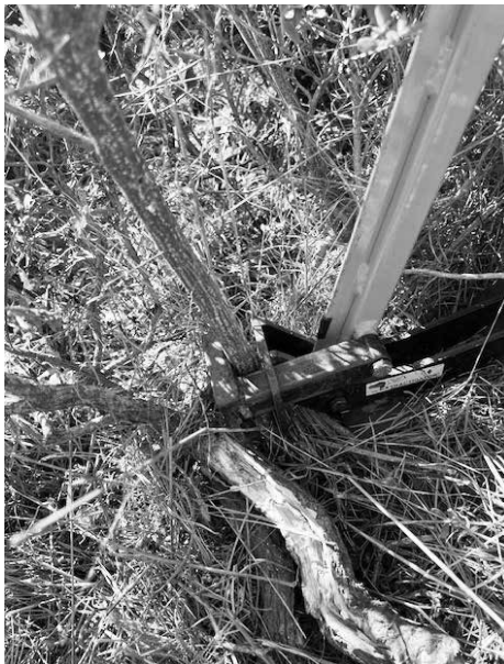
Position Weed Wrench around base of French broom plant
